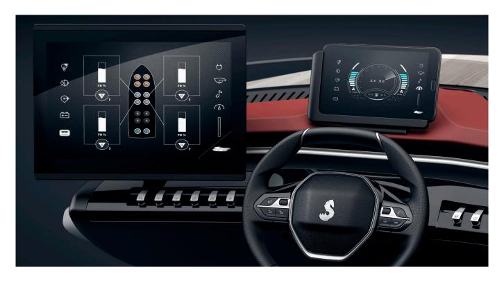
The Ship Control® interface is an onboard computer which assists in both navigation and life onboard the boat. Its connectivity allows the crew members to consult information about the boat: navigation, engine regime, control of the level of the batteries and reservoirs, air conditioning, lighting, and Hi-Fi.
