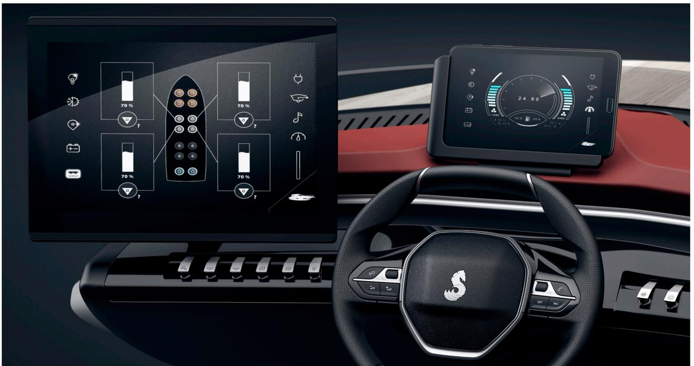
The Ship Control® interface is an onboard computer which assists in both navigation and life onboard the boat. Its connectivity allows the crew members to consult information about the boat: navigation, engine regime, control of the level of the batteries and reservoirs, air conditioning, lighting, and Hi-Fi.
