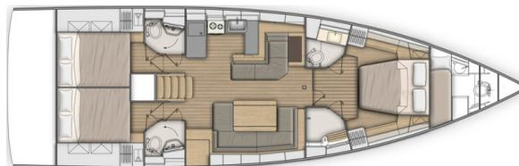
The pantry goes to the starboard side and is replaced by a head.
