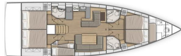
The starboard head of the standard version is replaced by a cabin with bunk beds:
